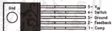
Figure 2. 5-Lead (Bent, Staggered Leads) TO-220 (T) – Top View See Package Number NDH0005D
