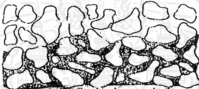
Moisture distribution in a particulate-solid bed during the second falling-rate period
