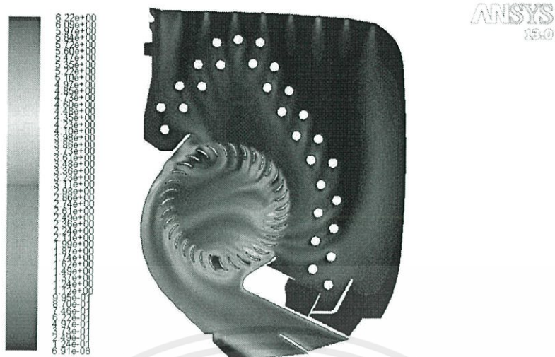
Contours of Turbulent Kinetic Energy (k) (m2/s2) Apr 11, 2014 ANSYS FLUENT 13.0 (2d, pbns, rke)
