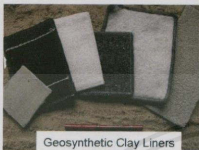
รูป 2.29 Geosynthetic clay liners(GCLs) [Research475 ,2014]
