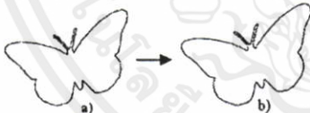
Fig. 3. The digitized contour smoothed by Gaussian filter a) The original contour b) The smoothed contour
