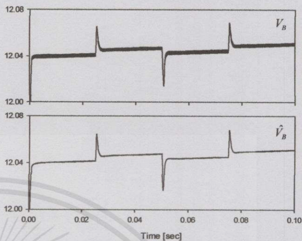
Fig. 7 Simulation result of battery voltage for step change of V_{sa-ref} from 42V to 38V
