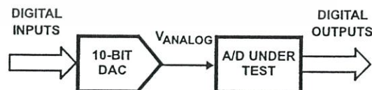
FIGURE 20. BASIC "DIGITAL" A/D TESTER
