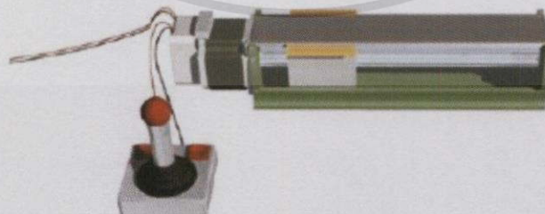
A slider system with V type Cool Muscle controlled by a joy stick
