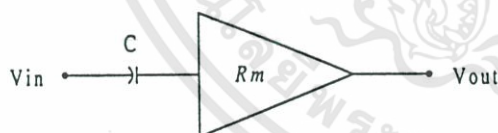
Fig. 1. The transresistance-capacitor ( R_m - C ) based differentiator
