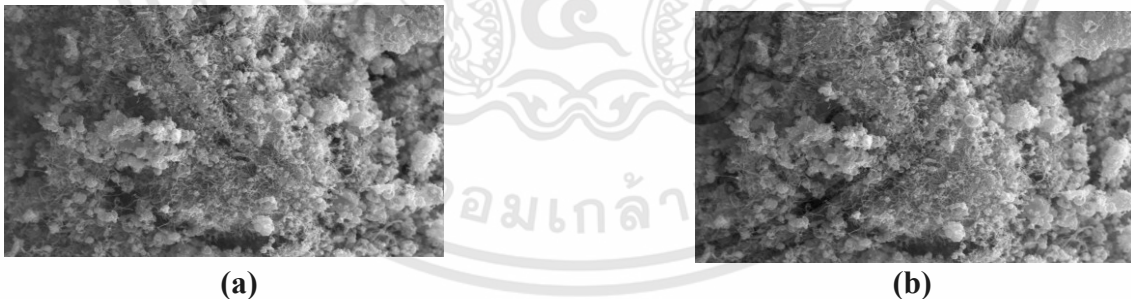
Figure 2 SEM images of SnO 2 /MWCNT nanocomposite using precursor concentration of 0.05 M under 300 W microwave irradiation (a) after irradiation (b) after calcination at 400°C.
