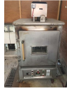
Fig. 2. PID temperature control electric oven
