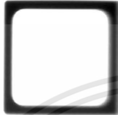
Fig. 5. The x-ray imaging of the aluminum hollow rectangle
