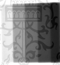
Fig. 10. The x-ray imaging of the aluminum step wedge
