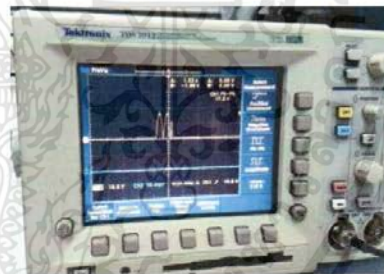
Figure 5 Digital oscilloscope capture the output of exposure time calibration (20 mSec)
