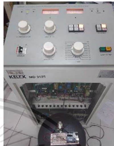
Fig. 4 Experimental set up for exposure time calibration
