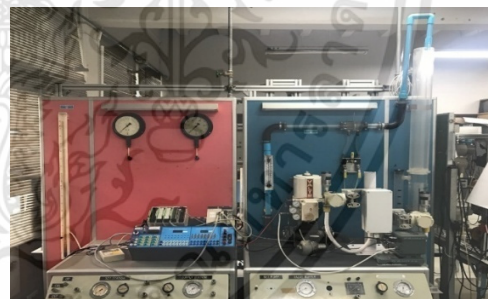
Fig. 9 The flow-level cascade controller.
