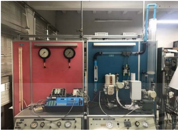
Fig. 3 Level control plant
