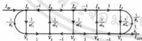
Fig. 6. SFG of fifth-order RLC low-pass filter prototype.
