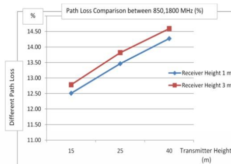
Fig. 10 The percentage different path loss in 850 MHz and 1800 MHz
