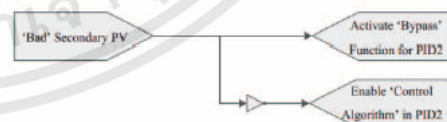
Figure 8. Logical concept to design the interlock for providing the control loop with high availability in analog system
