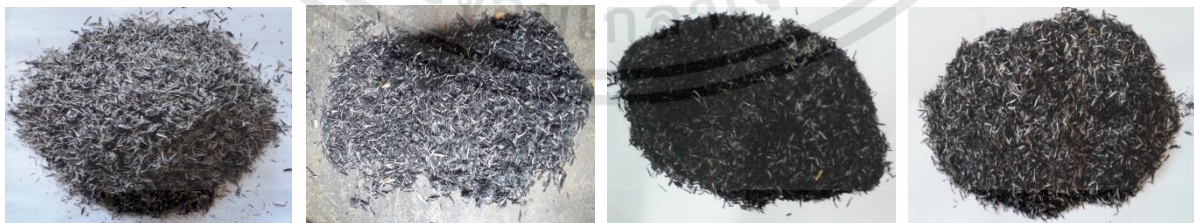
(a) Equivalence ratio 3.90 (b) Equivalence ratio 4.10 (c) Equivalence ratio 4.30 (d) Equivalence ratio 4.50
