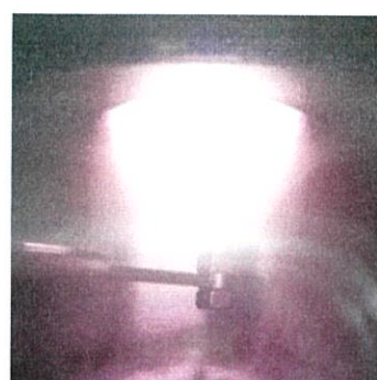
Ar flow rate = 40 sccm Voltage = 330 V
