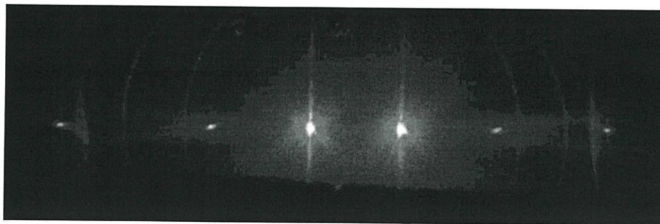
Figure 7. Higher orders of the anisotropic self diffraction up to third orders
