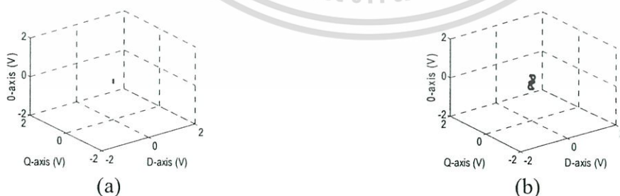
FIGURE 8. Patterns of dq0 voltage trajectory for, (a) balanced source, (b) healthy motor.
