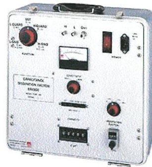
Transformer Ratio Arm bridge
