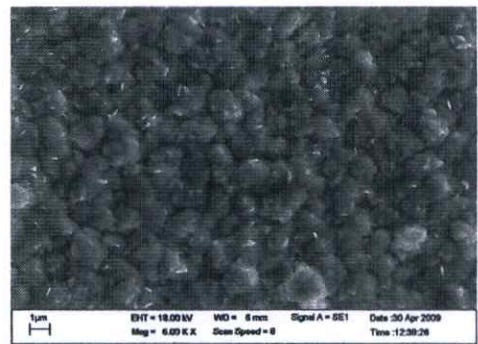
\text{Sb}_2\text{Te}_3/\text{Cu}/\text{slide glass}, T_{\text{sub}} = 100^\circ\text{C}
