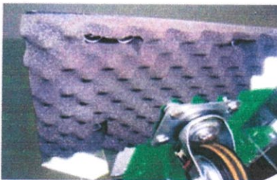
Figure 7. The acoustic sponge foam is mounted at the base of three ultrasonic sensors.
