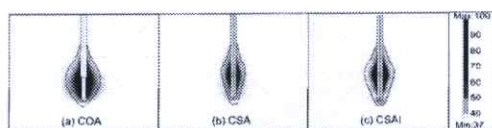
Fig. 5. Temperature distributions (50 W, 60 s) of single MW ablation from (a) COA (b) CSA, and (c) CSAI. The darkest regions in each case represent areas where temperature exceeds 50 °C. The dotted lines mark 60 °C contours.
