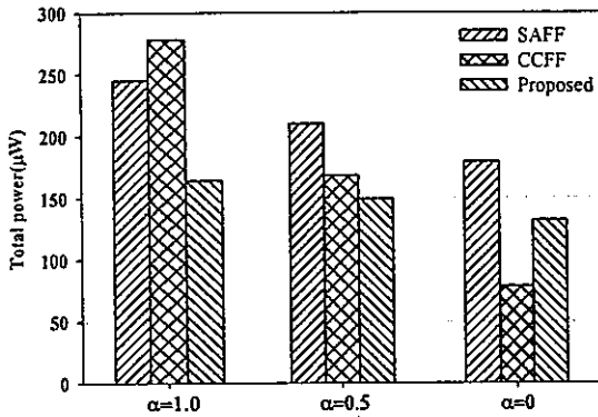
Fig.5: Power VS data switching activity at 400 MHz
