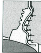
Seat after fire, with disc sealing load and line media pressure acting on the seat from the right. (Seat retainer upstream)
