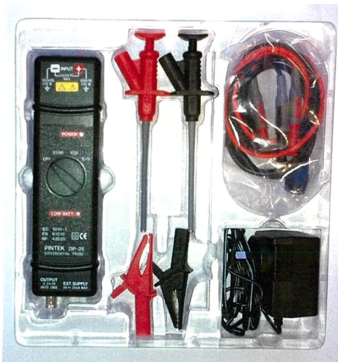
Differential Probe (PINTEK DP-25), 1000Vp, 25MHz
