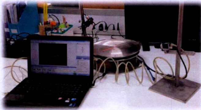
Figure 2 Inspection of Orifice Plate Flatness Using Laser Light Techniques System
