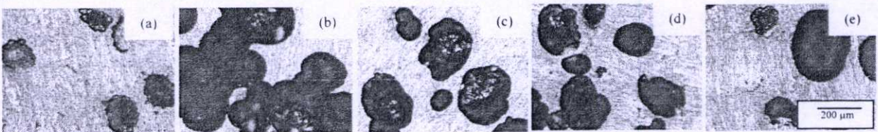
Figure. 6 AFM image of AAO nickel electroplating (a) 40°C, (b) 50°C, (c) 60°C with 30min, (d) 60 min, (e) 120 min with 50°C.
