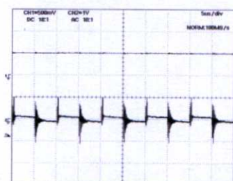
(a) x-scale: 5\mu\text{s}/\text{div} Top trace, I_o : y-scale: 0.5\text{A}/\text{div} Bottom trace, \Delta V_o : y-scale: 1\text{V}/\text{div}
