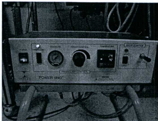
Figure 3.5 Snow dry-ice controller box
