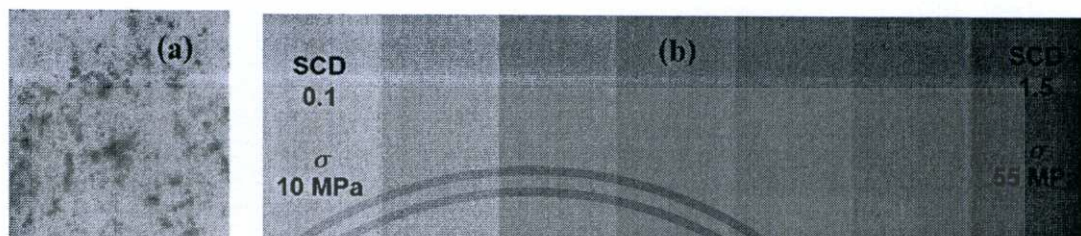
Figure 4.16 The red patches on Prescale sheets when pressure was applied (a) the standard momentary pressure chart (b)
