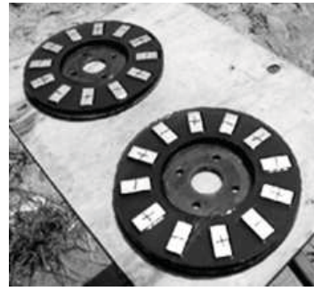
Fig. 2. Magnetic bars glued on two rotor disks
