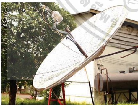
Fig. 14 the material on solar collector was acrylic mirror
