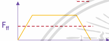
Friction feed-forward has additive effect on servo command at all times during move.
