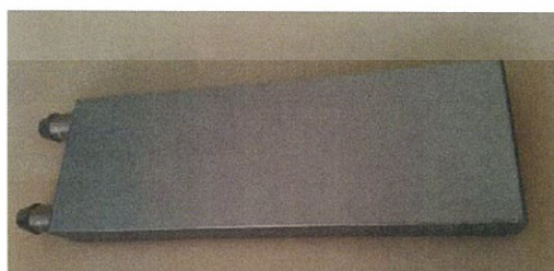
ข. Water cooling block
