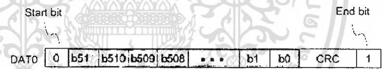
Data Packet Format for Standard Bus (only DAT0 used)
