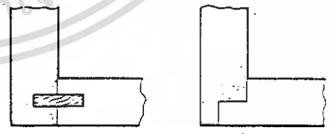
Butt joints between MDF panels
