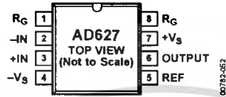
Figure 4. 8-Lead SOIC_N Pin Configuration
