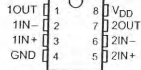
D, JG, P, OR PW PACKAGE (TOP VIEW)
