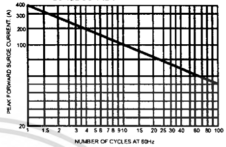
FIG. 2- MAXIMUM NON-REPETITIVE FORWARD SURGE CURRENT
