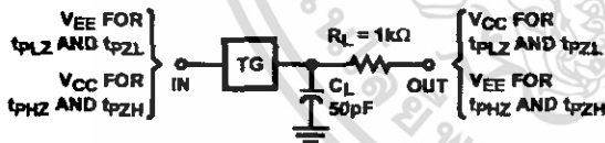
FIGURE 9. SWITCH ON/OFF PROPAGATION DELAY TEST CIRCUIT
