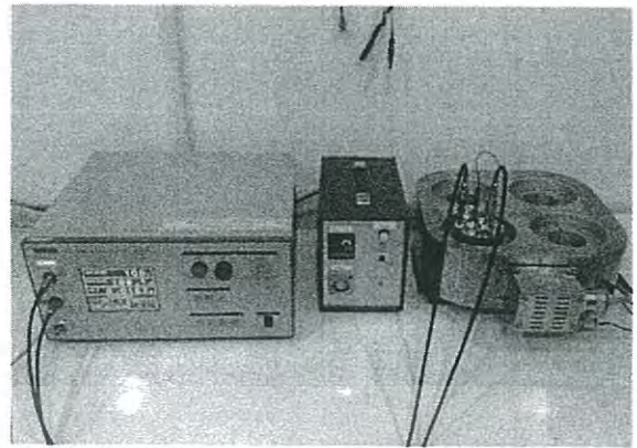
Fig. 5. C & tan \delta measurement
