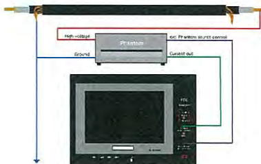
Fig. 6. Test circuit diagram for PDC measurement of XLPE cable with grounded shield
