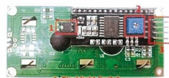
1. Blacklight Switch 2. Contrast Adjustment 3. I2C pin interface
