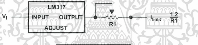
Figure 14. Precision Current-Limiter Circuit
