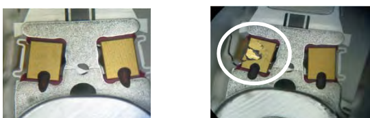
Fig.9 PZT element in working condition (left) and after a crack was introduced (right).
