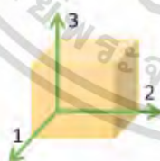
Fig. 3. Reference directions in a piezoelectric element
