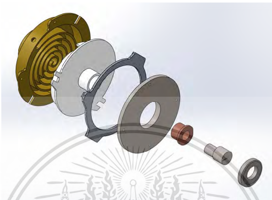
Fig. 4.23 Assembly of Scroll Expander model (bottom up)
