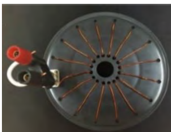
Fig. 8 The top view of the Rogowski coil.
