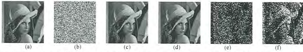
Figure 2. The decrypted image of lena color from (a) CML ( J=1 N=1 ), (b) CML ( J=7 N=7 ), (c) APCML ( J=1 N=1 ) and (d) APCML ( J=7 N=7 ). Show changed pixel of original for (e) CML ( J=1 N=1 ) and (f) CML ( J=7 N=7 ).
